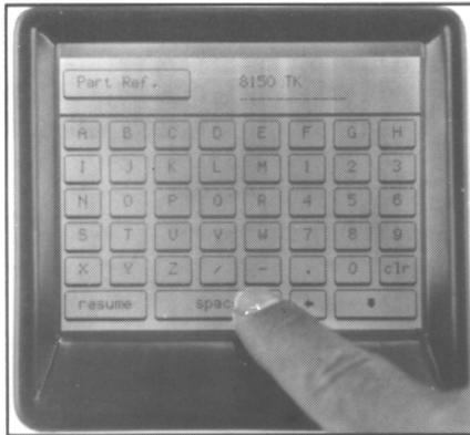
**Fig 3** Touchscreen on the latest Rockwell-type tester. A full alphanumeric keypad enables highly detailed identifying data to be stored and analysed
