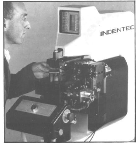
**Fig 5** Modern hardness testers can be engineered for use in unmanned test cells, providing data automatically for the host computer
