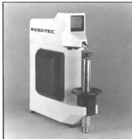
Fig 1 The latest Rockwell-type machines can analyse and communicate test data in a way compatible with effective SPC
