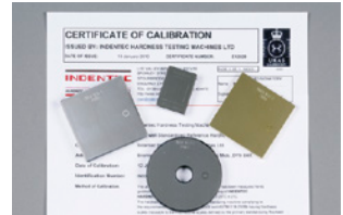
Hardness comparison plate with certificate
